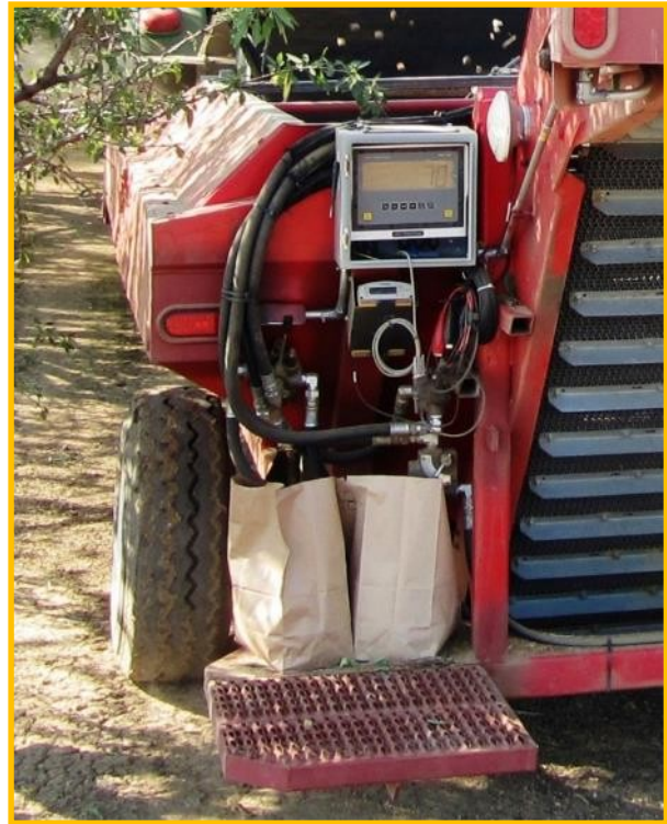
Trimble GPS acts as datalogger to collect continuous yield data
