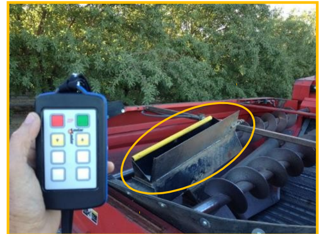
Wireless controller for hydraulically operated auto sampler
