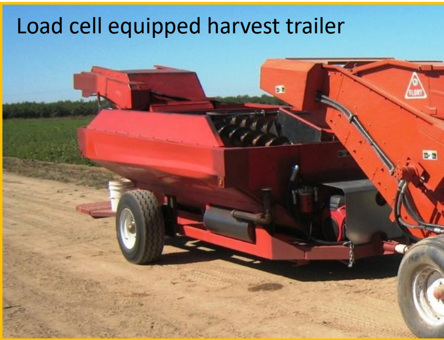
Self contained hydraulic system for operating augers, autosampler and elevator
