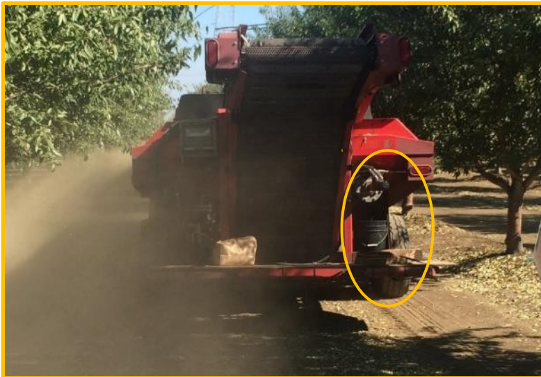
Autosampler delivers nuts to right rear of cart
